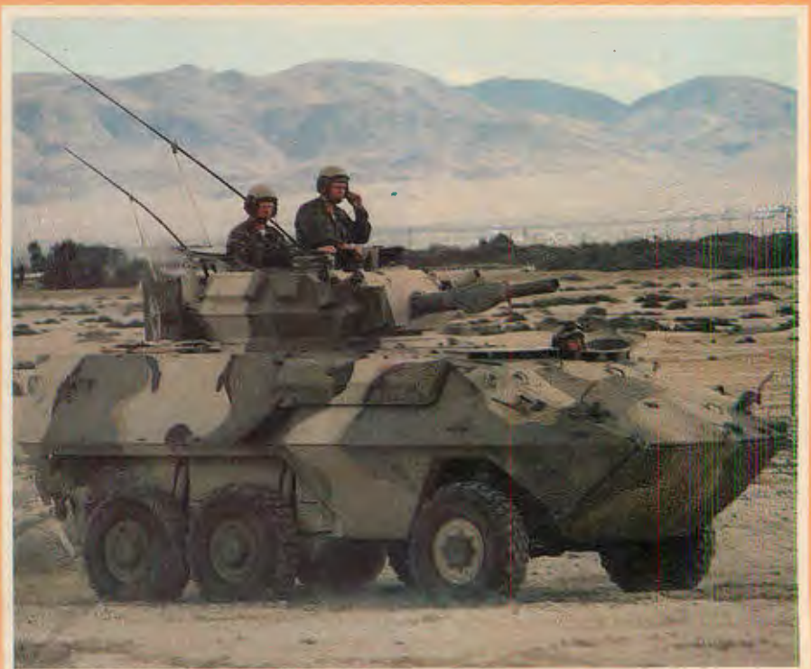
ABOVE: Cougar with 76mm gun and smoke-grenade launchers.
